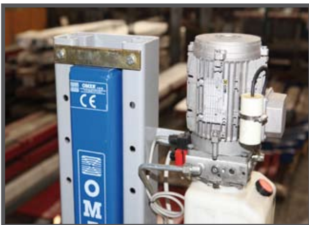
The vertical lifting height of the platform is set during the initial installation by means of locking steel plates mounted at the top of the columns, thus guaranteeing safety and determining the peak lifting height, designed to customer requirements and environment.
