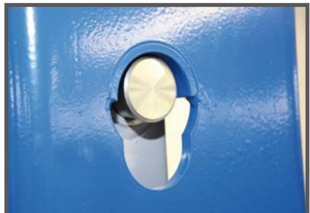
Detail of floor level mechanical locking device.
