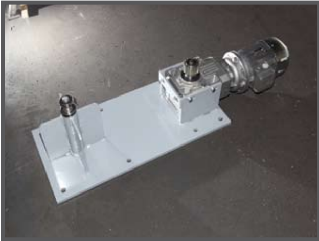
The gearmotor assembly - with central rotation pin and rotation pinion - is connected to the circular rack.
