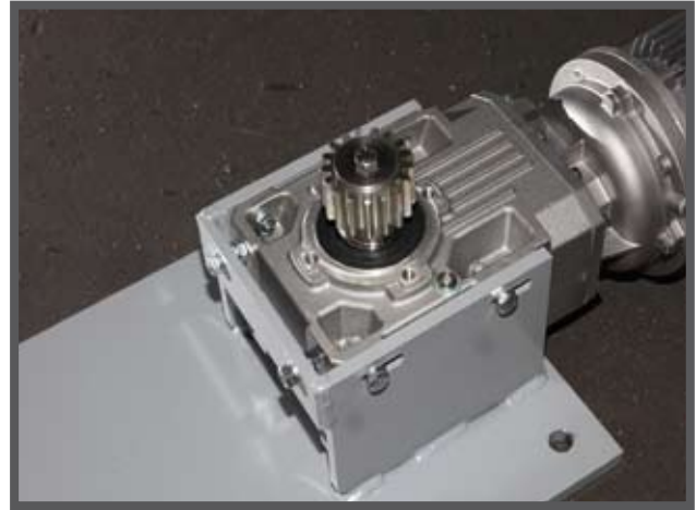
Detail of the gearmotor with rotation pinion. This photo shows the slots, fit with securing bolts, set on both the front (for right - left adjustment) and on the side (for forward - back adjustment).
