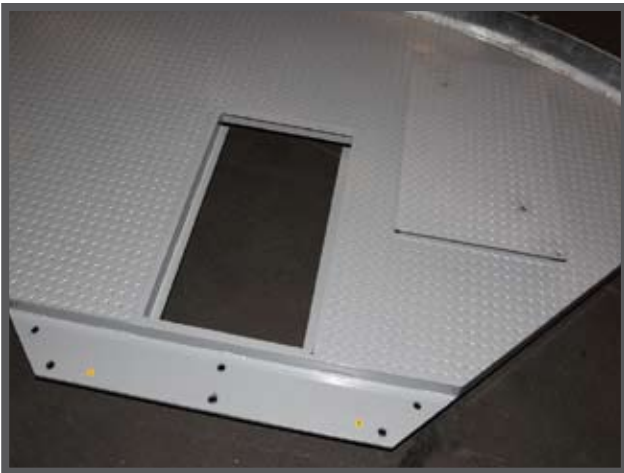
One of the four sections has a hatch for inspection of the motor and for maintenance.
