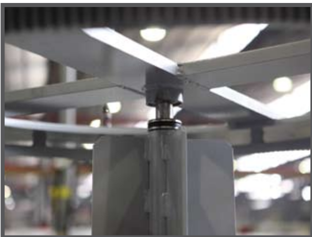
The connection structure is snapped into the central rotation pin in the underlying area.
