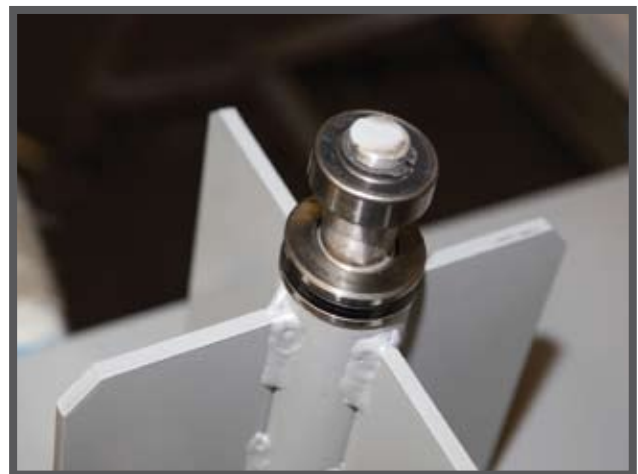
The central rotation pin - set on the motor assembly and fit with thrust bearings to completely absorb compression due to weight - is used to accommodate the connection structure.
